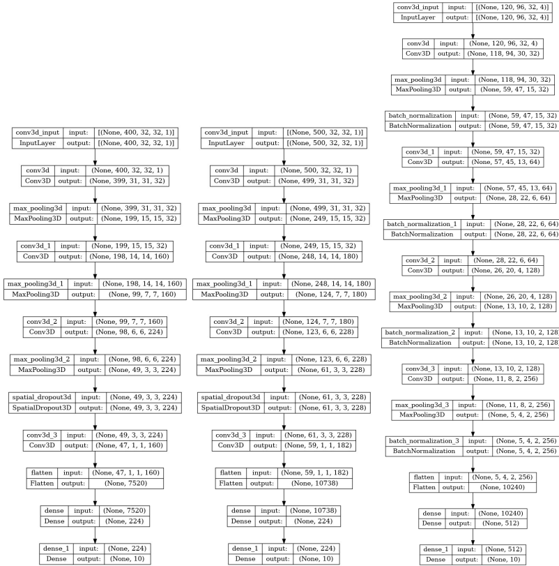
Fig. 5 Model architectures for Range-Angles —left, Range-Doppler —centre and IQ —right
